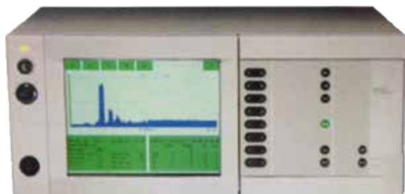
Controlli difetti superficiali in linea 100% eddy-current testing on surface wire for quality assurance
